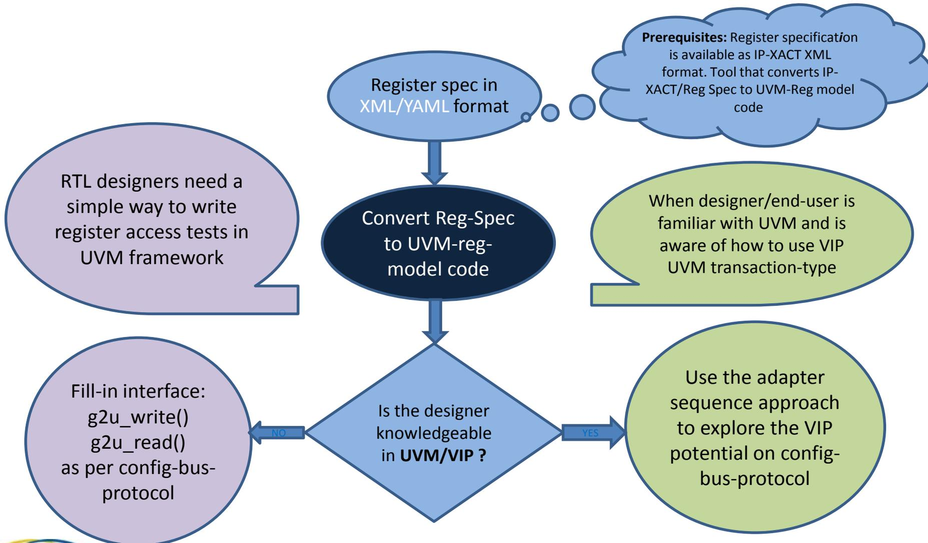
**Prerequisites:** Register specification is available as IP-XACT XML format. Tool that converts IP-XACT/Reg Spec to UVM-Reg model code
